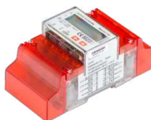
Meter 3f PR0380-Mb x/5A M-Bus Three-phase electricity meter indirect measurement, MID approved. Pulses & M-Bus data output - 3×230V/400V, 100A.
