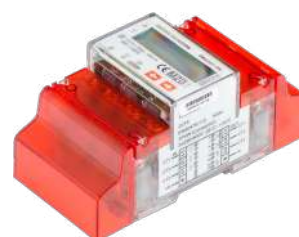
Meter 3f PR0380-Mb 100A M-Bus Three-phase 380V M-Bus energy meter for direct measuring (max load 100A). Pulses & M-Bus data output - 3×230V/400V, 100A.
