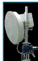
Tracking dish antenna
