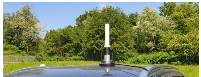
omni antenna with magnetic support for mobile operations
