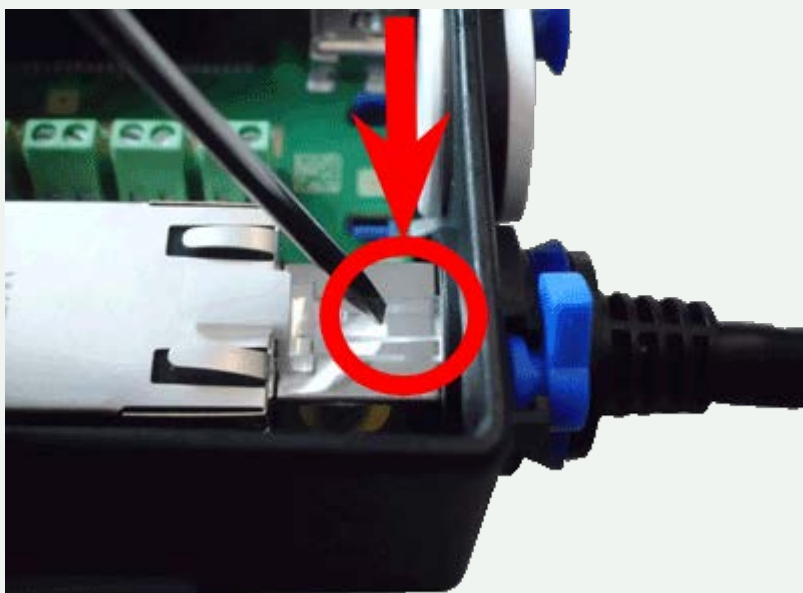
Fig. 16: Hold down clip when removing the network connector from the box!
