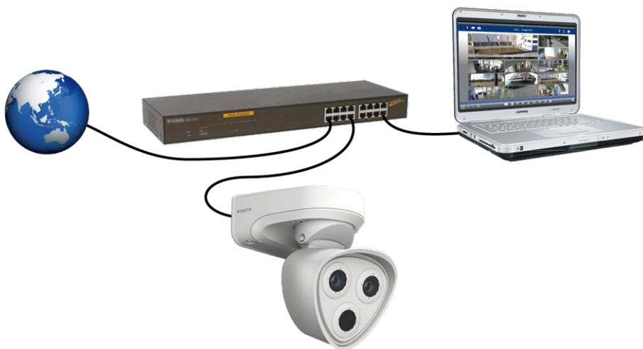
Fig. 13: Power supply using PoE switch according to PoE Plus (802.3at-2009)
